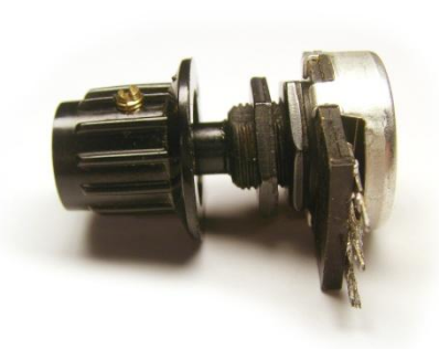
Figure 7-4: Potentiometer with knob
