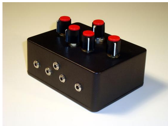
Figure 7-5: Potentiometer knobs on electronic device 18
