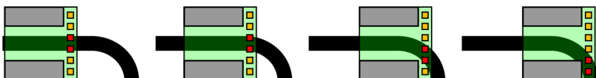
Figure 11-9: Changing line position as robot drives forwards
