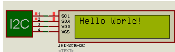
Figure 4-6: "Hello World!" displayed on LCD
