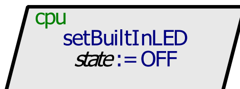
Figure 2-22: setBuiltInLED routine with "state" set to "OFF"
