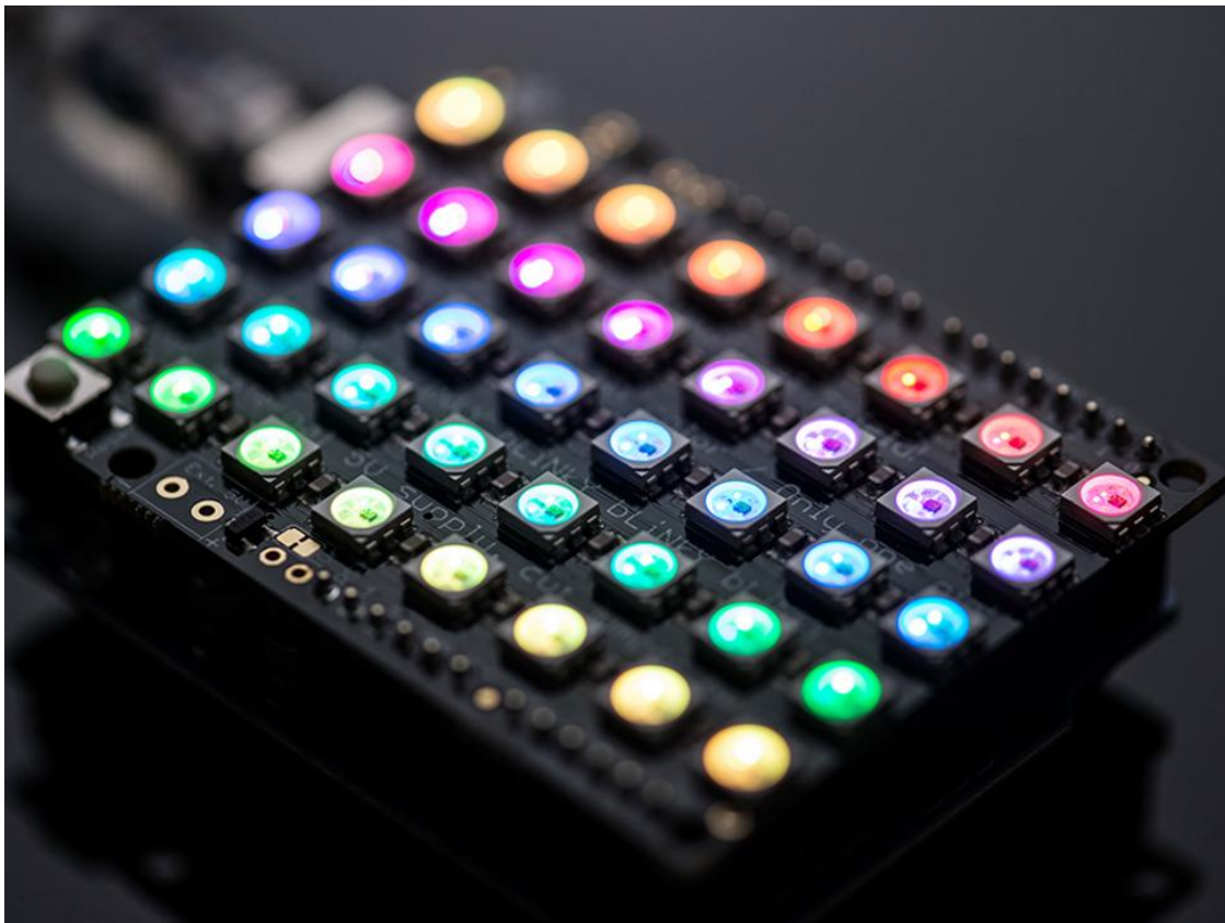
Figure 8-1: Adafruit NeoPixel shield for Arduino 20
